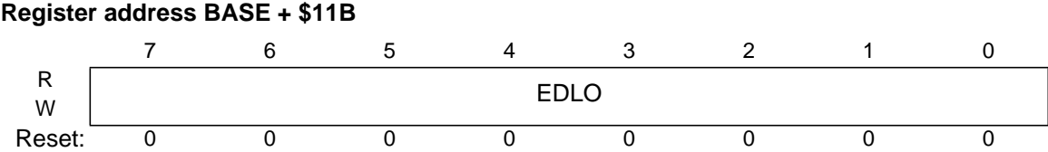
Figure 3-13 EEPROM Data Low Register (EDATALO)
