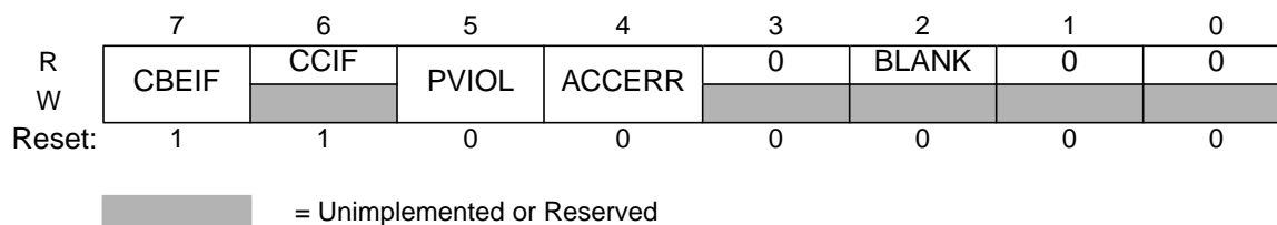
Figure 3-7 EEPROM Status Register (ESTAT)
