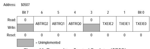
Figure 22. Transmitter Control Register (CTCR)
