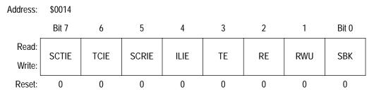
Figure 12. SCI Control Register 2 (SCC2)
