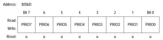
Figure 13. Transmit Buffer Priority Register (TBPR)
