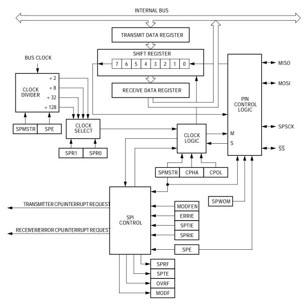
Figure 1. SPI Module Block Diagram
