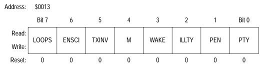
Figure 11. SCI Control Register 1 (SCC1)
