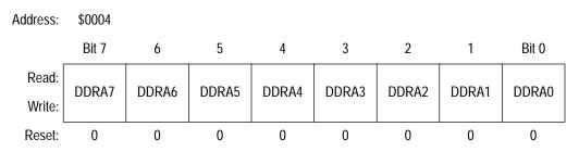
Figure 3. Data Direction Register A (DDRA)
