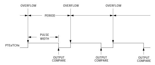
Figure 3. PWM Period and Pulse Width
