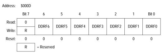
Figure 18. Data Direction Register F (DDRF)
