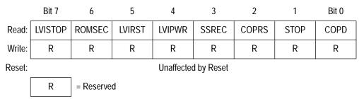
Figure 1. Configuration Register (CONFIG-1)
