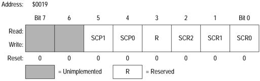
Figure 18. SCI Baud Rate Register (SCBR)
