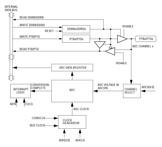
Figure 1. ADC Block Diagram
