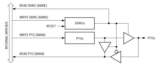
Figure 22. Port G I/O Circuit
