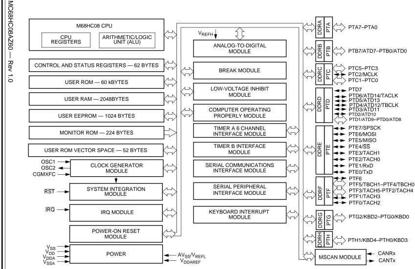
Figure 1. MCU Block Diagram for the MC68HC08AZ60 (64-Pin QFP)
