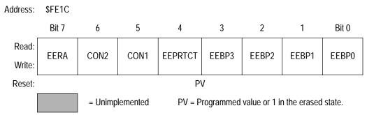
Figure 2. EEPROM-1 Nonvolatile Register (EENVR1)
