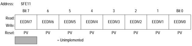
Figure 6. EEPROM-2 Divider Low Non-volatile Register (EEDIVLNVR)
