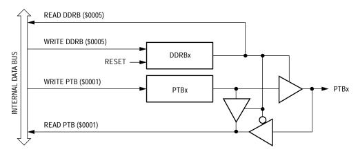
Figure 7. Port B I/O Circuit
