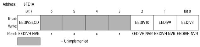
Figure 3. EEPROM-2 Divider High Register (EEDIVH)
