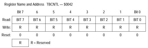
Figure 5. TIMB Counter Registers (TBCNTH and TBCNTL)
