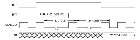
Figure 5. Internal Reset Timing
