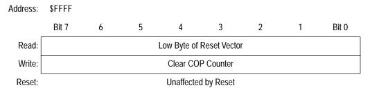
Figure 2. COP Control Register (COPCTL)
