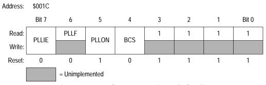
Figure 4. PLL Control Register (PCTL)
