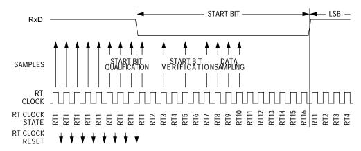
Figure 8. Receiver Data Sampling
