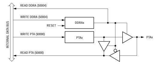
Figure 4. Port A I/O Circuit
