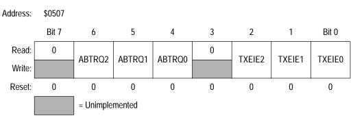
Figure 22. Transmitter Control Register (CTCR)
