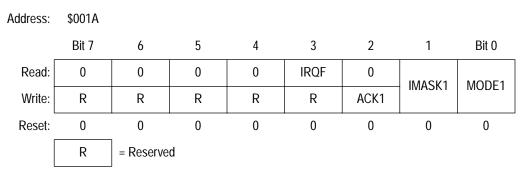
Figure 3. IRQ Status and Control Register (ISCR)
