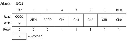
Figure 2. ADC Status and Control Register (ADSCR)
