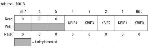
Figure 4. Keyboard Interrupt Enable Register (KBIER)
