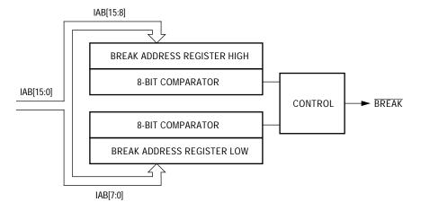
Figure 1. Break Module Block Diagram
