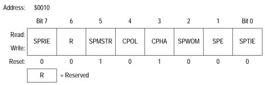
Figure 11. SPI Control Register (SPCR)
