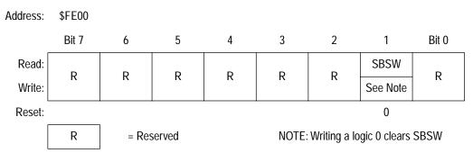
Figure 17. SIM Break Status Register (SBSR)
