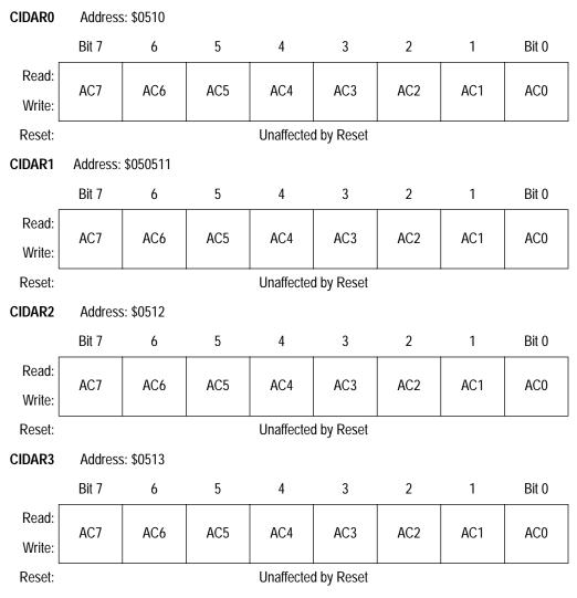
Figure 26. Identifier Acceptance Registers (CIDAR0-CIDAR3)
