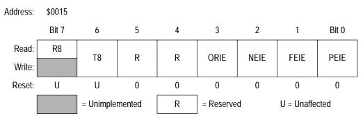
Figure 13. SCI Control Register 3 (SCC3)
