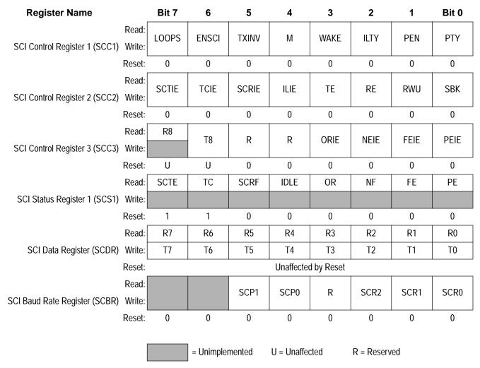
Figure 5. SCI Transmitter I/O Register Summary
