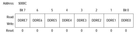
Figure 15. Data Direction Register E (DDRE)
