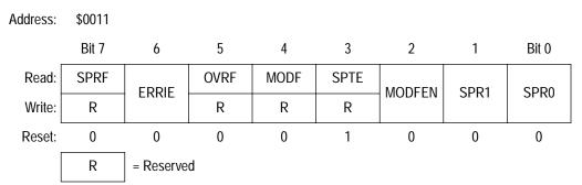
Figure 12. SPI Status and Control Register (SPSCR)
