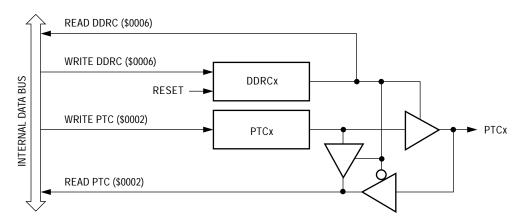
Figure 10. Port C I/O Circuit
