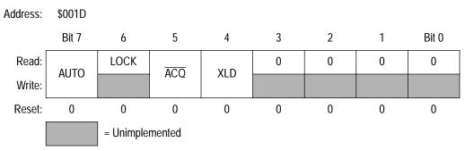
Figure 5. PLL Bandwidth Control Register (PBWC)
