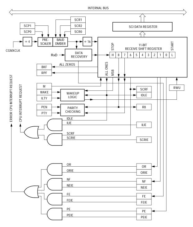
Figure 6. SCI Receiver Block Diagram
