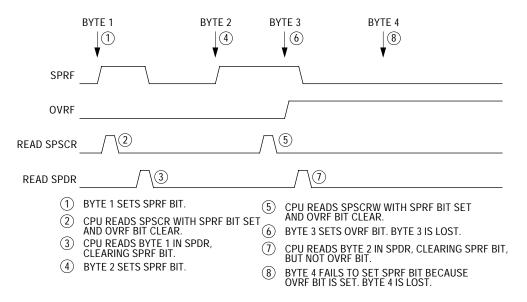
Figure 6. Missed Read of Overflow Condition
