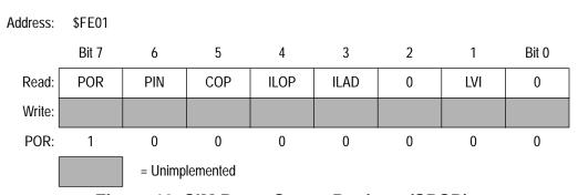
Figure 18. SIM Reset Status Register (SRSR)
