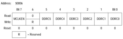
Figure 9. Data Direction Register C (DDRC)
