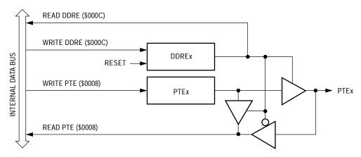
Figure 16. Port E I/O Circuit
