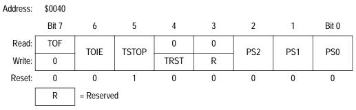
Figure 4. TIMB Status and Control Register (TBSC)
