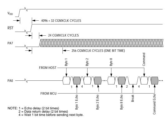
Figure 6. Monitor Mode Entry Timing
