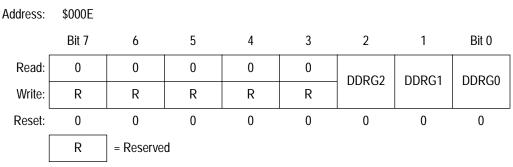
Figure 21. Data Direction Register G (DDRG)
