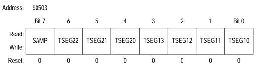
Figure 18. Bus Timing Register 1 (CBTR1)
