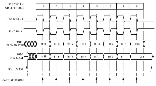
Figure 4. Transmission Format (CPHA = 1)
