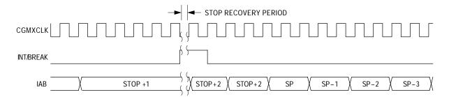
Figure 16. Stop Mode Recovery from Interrupt or Break
