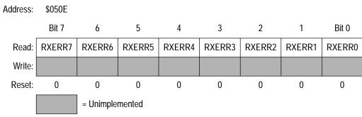
Figure 24. Receiver Error Counter (CRXERR)
