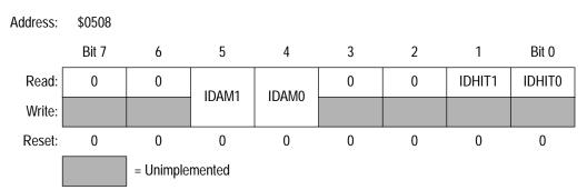
Figure 23. Identifier Acceptance Control Register (CIDAC)
