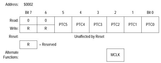
Figure 8. Port C Data Register (PTC)
