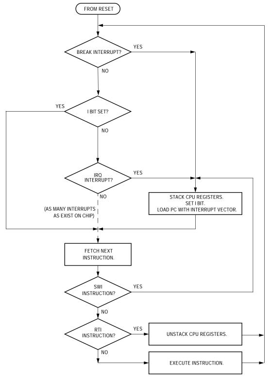
Figure 9. Interrupt Processing
