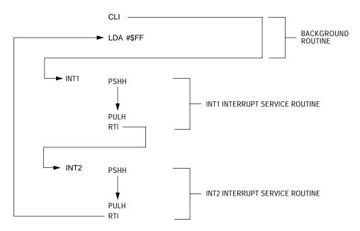
Figure 11. Interrupt Recognition Example
