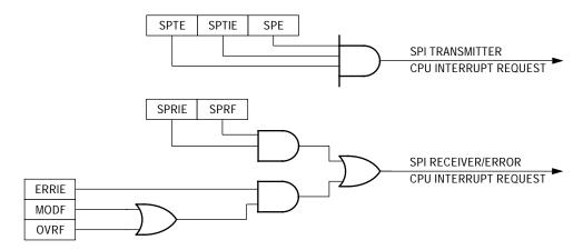
Figure 8. SPI Interrupt Request Generation
