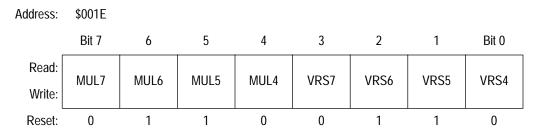
Figure 6. PLL Programming Register (PPG)
