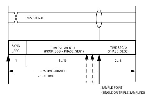
Figure 8. Segments within the Bit Time
