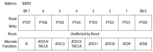
Figure 11. Port D Data Register (PTD)
