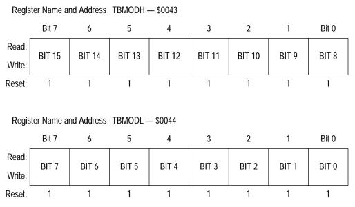
Figure 6. TIMB Counter Modulo Registers (TMODH and TMODL)
