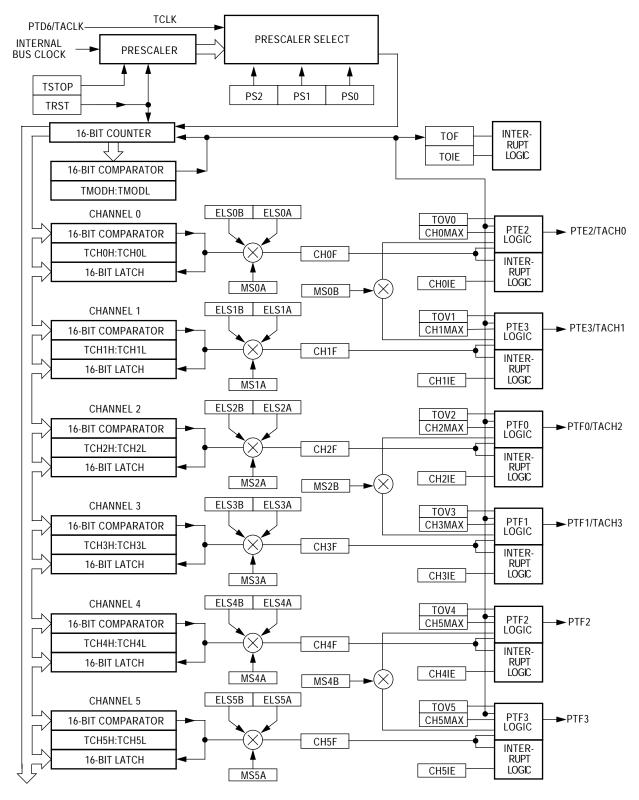
Figure 1. TIMA Block Diagram
