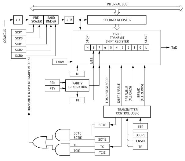
Figure 4. SCI Transmitter
