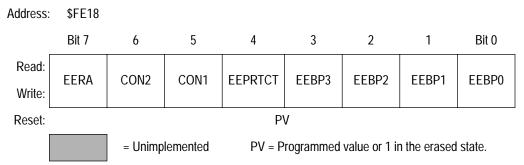
Figure 2. EEPROM-2 Nonvolatile Register (EENVR2)
