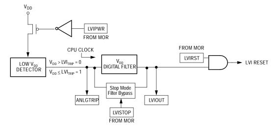
Figure 1. LVI Module Block Diagram
