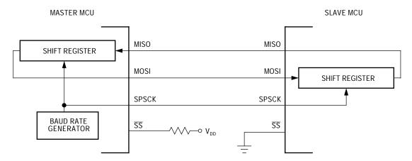
Figure 2. Full-Duplex Master-Slave Connections
