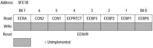
Figure 3. EEPROM-2 Array Control Register (EEACR2)
