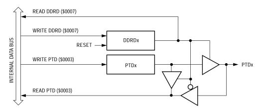
Figure 13. Port D I/O Circuit
