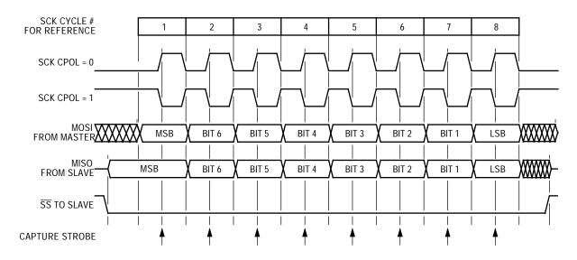
Figure 3. Transmission Format (CPHA = 0)
