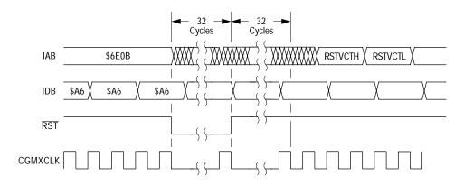
Figure 14. Wait Recovery from Internal Reset
