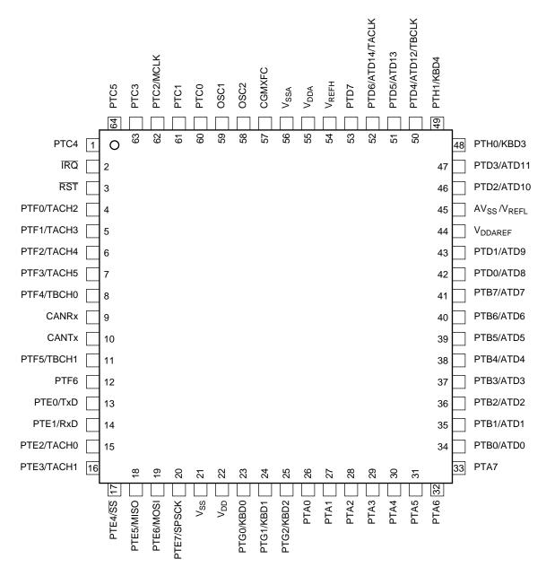
Figure 2. MC68HC08AZ60 (64-Pin QFP)
