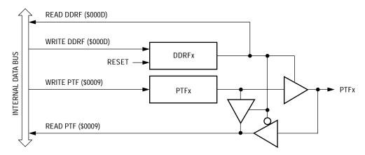
Figure 19. Port F I/O Circuit
