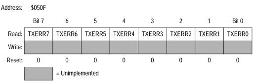
**Figure 25. Transmit Error Counter (CTXERR)**
