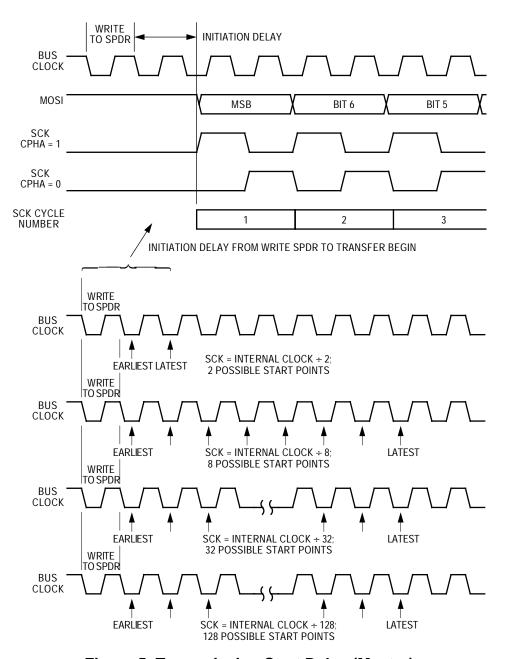
Figure 5. Transmission Start Delay (Master)
