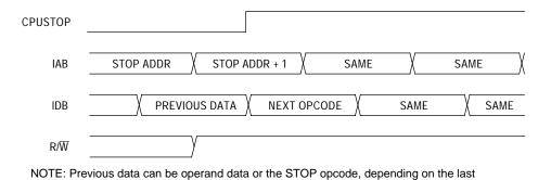
Figure 15. Stop Mode Entry Timing
