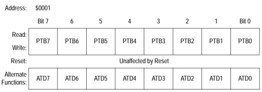
Figure 5. Port B Data Register (PTB)
