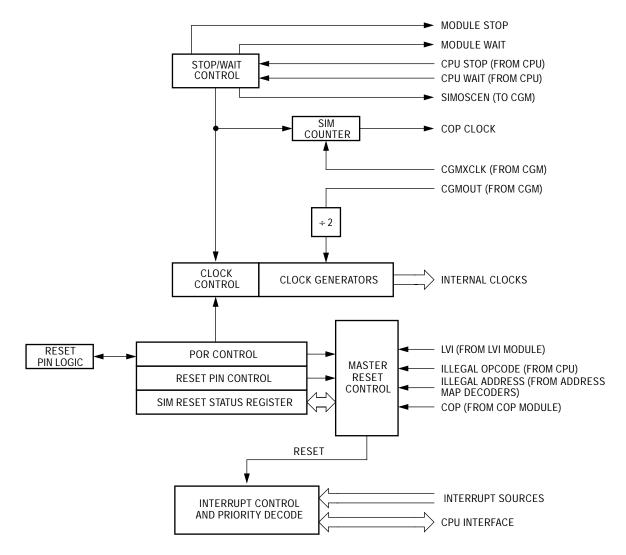
Figure 1. SIM Block Diagram
