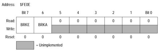
Figure 3. Break Status and Control Register (BSCR)
