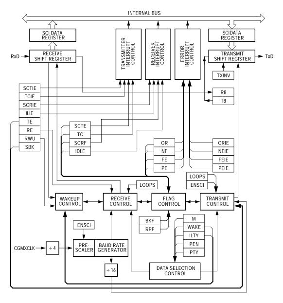
Figure 1. SCI Module Block Diagram
