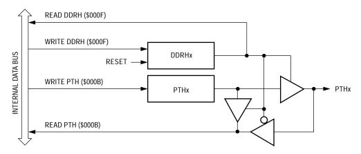
Figure 25. Port H I/O Circuit
