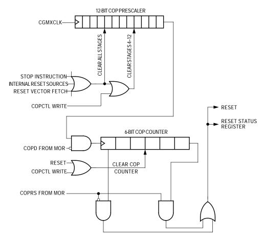
Figure 1. COP Block Diagram
