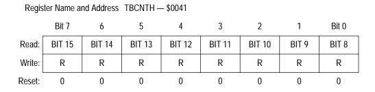
Figure 5. TIMB Counter Registers (TBCNTH and TBCNTL)
