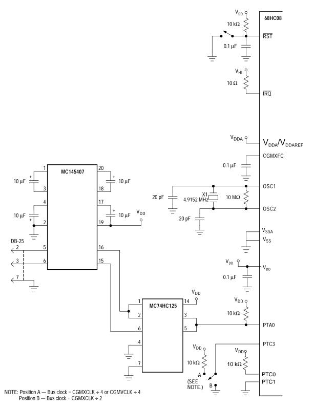
**Figure 1. Monitor Mode Circuit**
