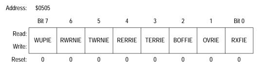
Figure 20. Receiver Interrupt Enable Register (CRIER)
