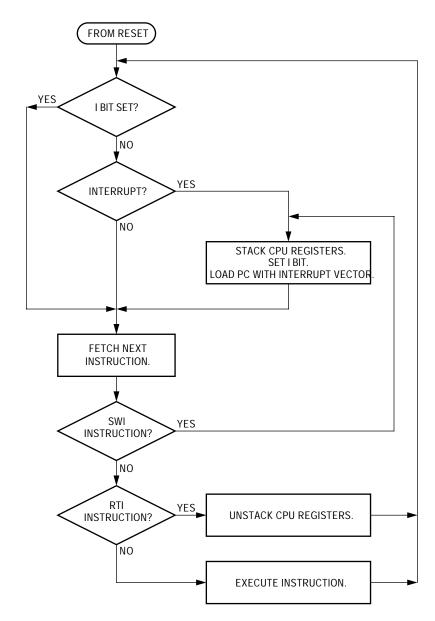
Figure 2. IRQ Interrupt Flowchart
