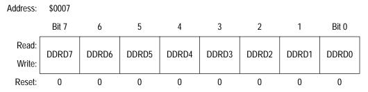
Figure 12. Data Direction Register D (DDRD)
