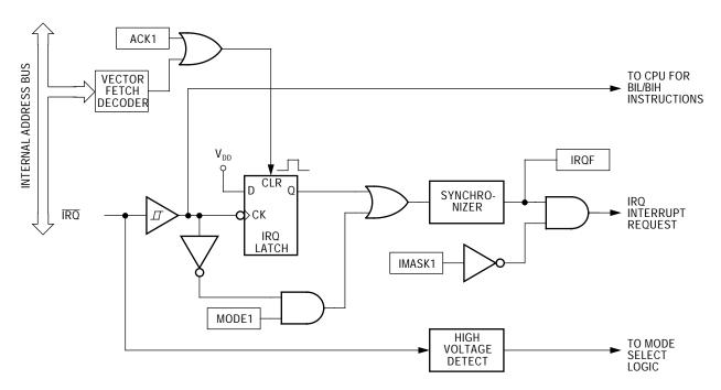
Figure 1. IRQ Block Diagram
