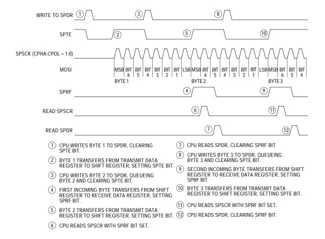
Figure 9. SPRF/SPTE CPU Interrupt Timing
