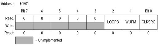
Figure 16. Module Control Register (CMCR1)
