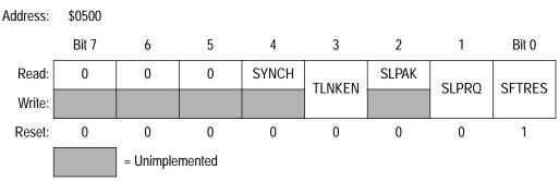
Figure 15. Module Control Register 0 (CMCR0)
