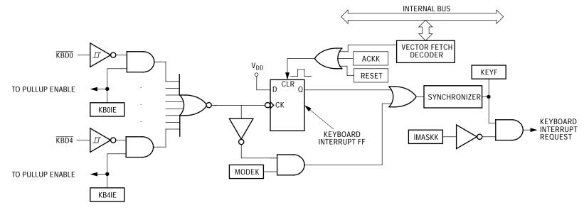
Figure 1. Keyboard Module Block Diagram
