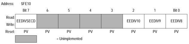
Figure 5. EEPROM-2 Divider High Non-volatile Register (EEDIVHNVR)
