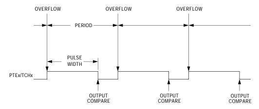
Figure 3. PWM Period and Pulse Width
