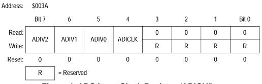
Figure 4. ADC Input Clock Register (ADICLK)
