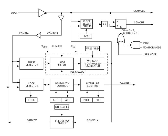
Figure 1. CGM Block Diagram
