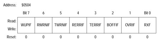
Figure 19. Receiver Flag Register (CRFLG)
