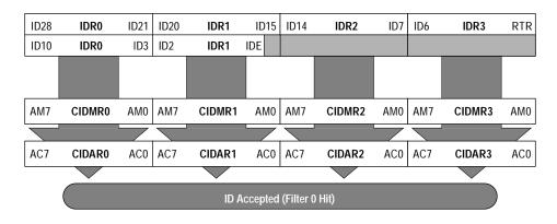
Figure 3. Single 32-Bit Maskable Identifier Acceptance Filter
