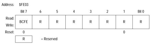
Figure 19. SIM Break Flag Control Register (SBFCR)
