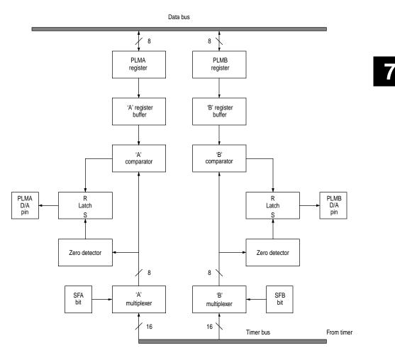
Figure 7-1 PLM system block diagram
