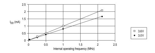
Figure 11-8 Run I<sub>DD</sub> vs internal operating frequency (3 V, 3.6 V)
