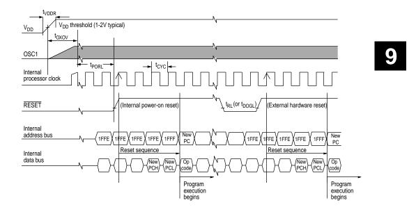
Figure 9-1 Reset timing diagram
