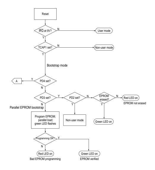
Figure C-3 Modes of operation flow chart (1 of 2)
