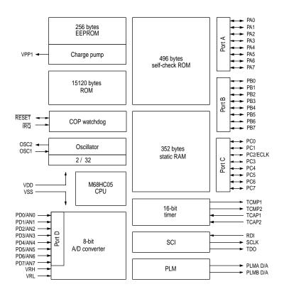
Figure D-1 MC68HC05B16 block diagram
