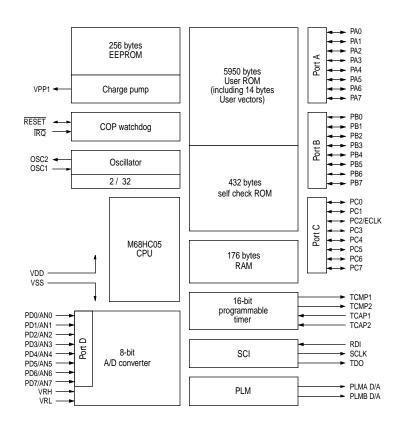
Figure 1-1 MC68HC05B6 block diagram
