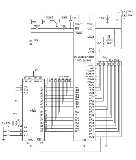
Figure E-10 RAM parallel bootstrap schematic diagram
