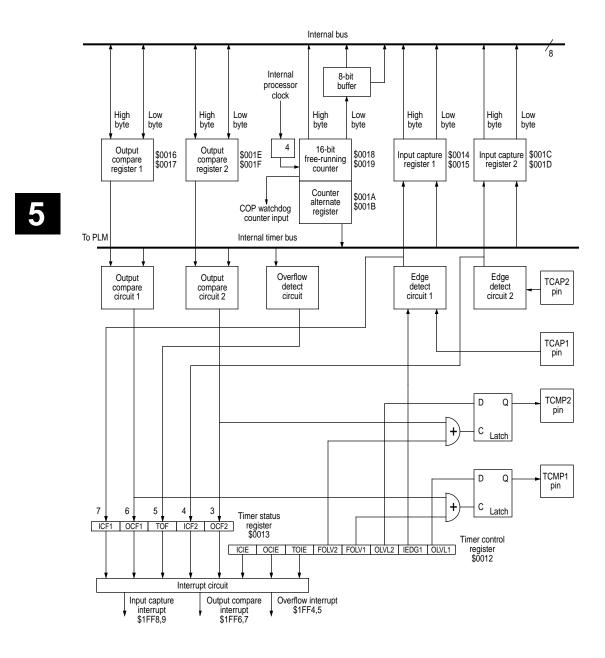
Figure 5-1 16-bit programmable timer block diagram
