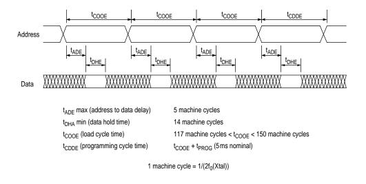
Figure C-9 EPROM parallel bootstrap loader timing diagram
