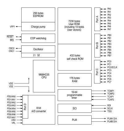
Figure B-1 MC68HC05B8 block diagram
