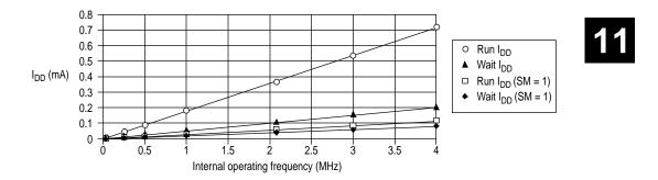
Figure 11-7  $I_{DD}$  vs mode vs internal operating frequency,  $V_{DD}$  = 5.5V
