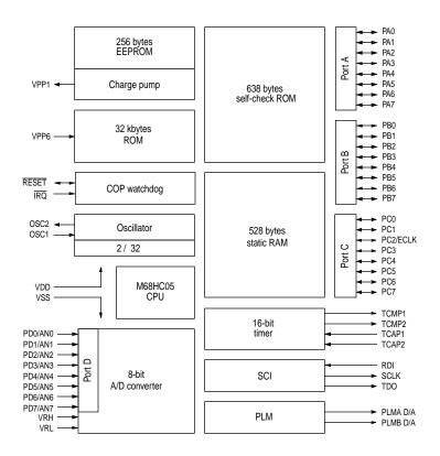
Figure F-1 MC68HC05B32 block diagram
