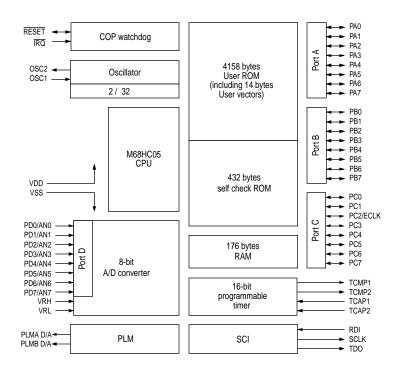
Figure A-1 MC68HC05B4 block diagram
