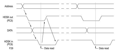
Figure C-5 Timing diagram with handshake
