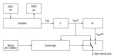
Figure 2-5 Slow mode divider block diagram
