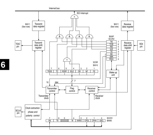
*Note:* The serial communications data register (SCI SCDR) is controlled by the internal  $R/\overline{W}$  signal. It is the transmit data register when written to and the receive data register when read.
