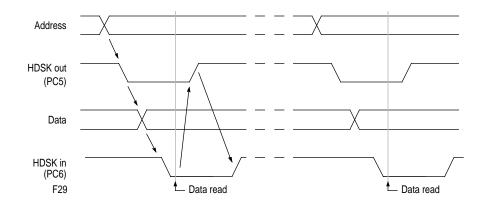
Figure G-5 Timing diagram with handshake
