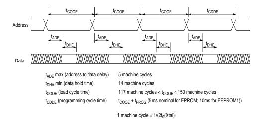
Figure G-6 Parallel EPROM loader timing diagram
