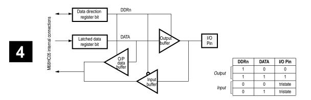
Figure 4-1 Standard I/O port structure
