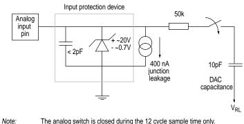
The analog switch is closed during the 12 cycle sample time only.
