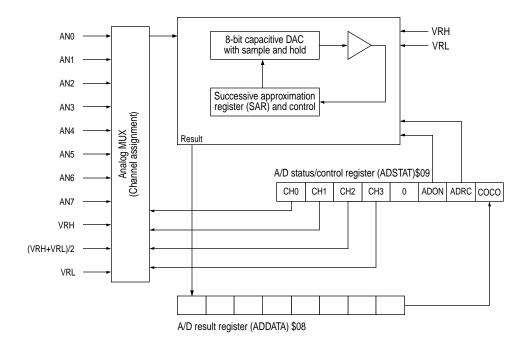
Figure 8-1 A/D converter block diagram
