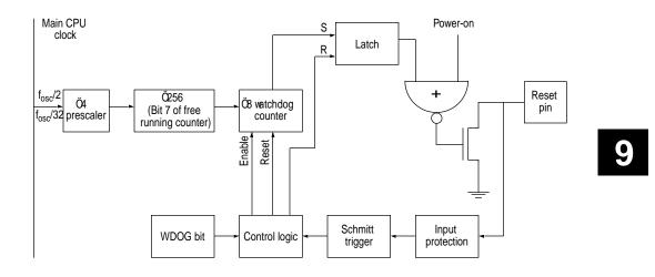
Figure 9-2 Watchdog system block diagram
