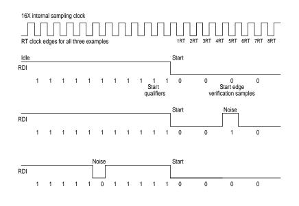
Figure 6-4 SCI examples of start bit sampling technique
