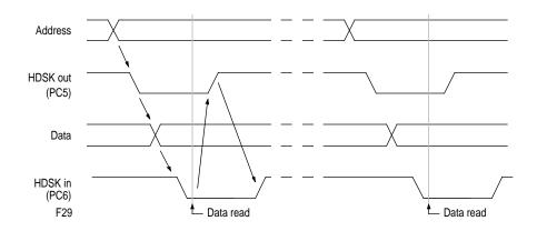
Figure E-5 Timing diagram with handshake
