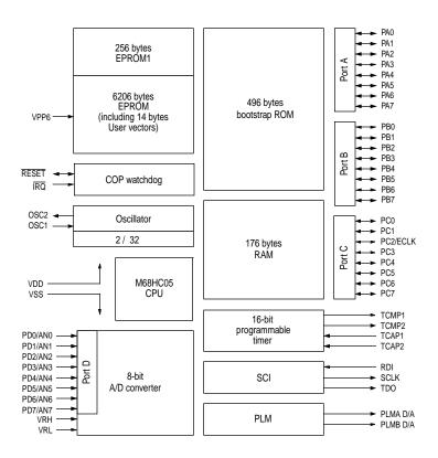
Figure C-1 MC68HC705B5 block diagram
