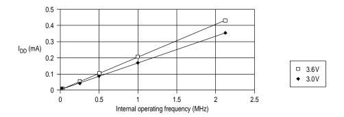
Figure 11-11 Wait  $I_{DD}$  (SM = 1) vs internal operating frequency (3V, 3.6V)
