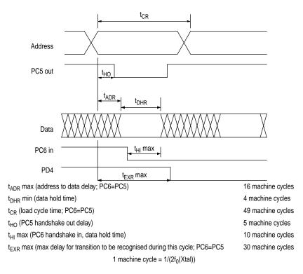
Figure E-9 Parallel RAM loader timing diagram
