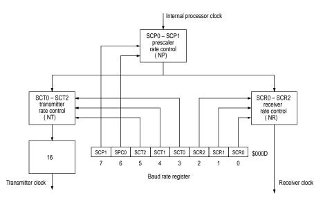
Note: There is a fixed rate divide-by-16 before the transmitter to compensate for the inherent divide-by-16 of the receiver (sampling). This means that by loading the same value for both the transmitter and receiver baud rate selector, the same baud rates can be obtained.
