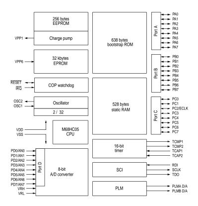
Figure G-1 MC68HC705B32 block diagram
