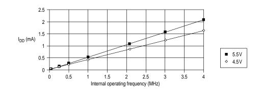
Figure 11-4 Wait I<sub>DD</sub> vs internal operating frequency (4.5V, 5.5V)
