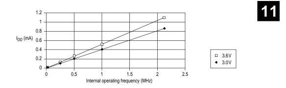
Figure 11-10 Wait  $I_{DD}$  vs internal operating frequency (3V, 3.6V)
