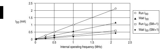
Figure 11-13  $I_{DD}$  vs mode vs internal operating frequency,  $V_{DD}$  = 3.6V
