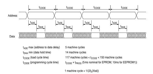
Figure E-6 Parallel EPROM loader timing diagram
