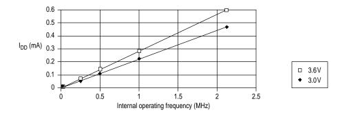
Figure 11-9 Run  $I_{DD}$  (SM = 1) vs internal operating frequency (3V,3.6V)
