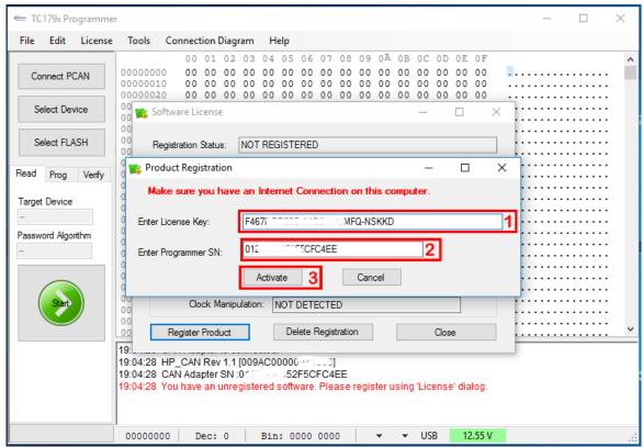
Figure 21 TC179x-Programmer software activation
