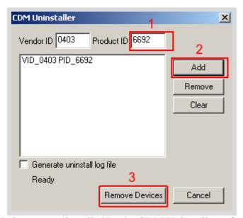
Figure 19 The Drivers are uninstalled by the CDM Uninstaller software
