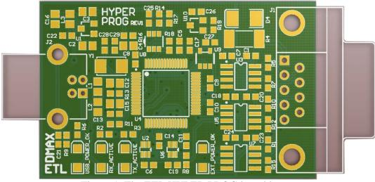
Figure 1. The ETL HYPER PROG board layout
