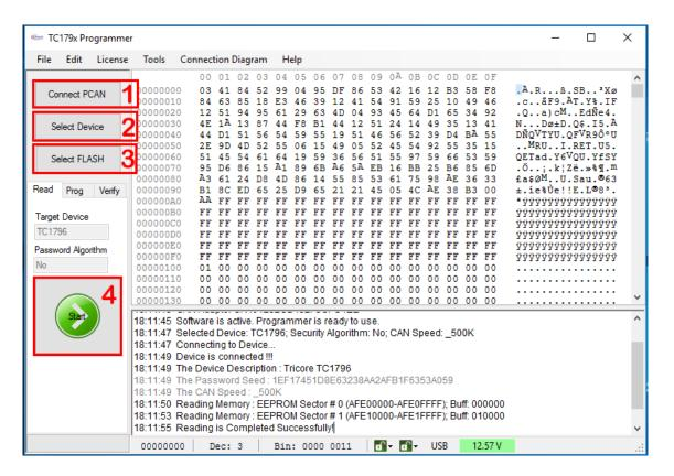
Figure 26 TC179x-Programmer reading sequence.
