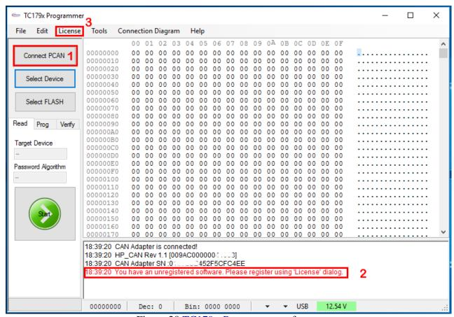
Figure 20 TC179x-Programmer software
