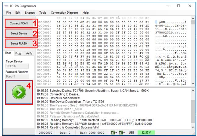
Figure 28 TC179x-Programmer reading sequence.
