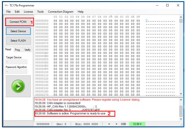
Figure 23 Successful TC179x-Programmer activation and connection
