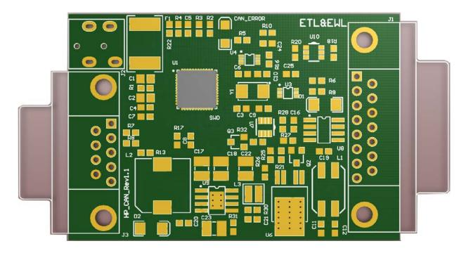
Figure 2. The ETL HP CAN adapter board layout
