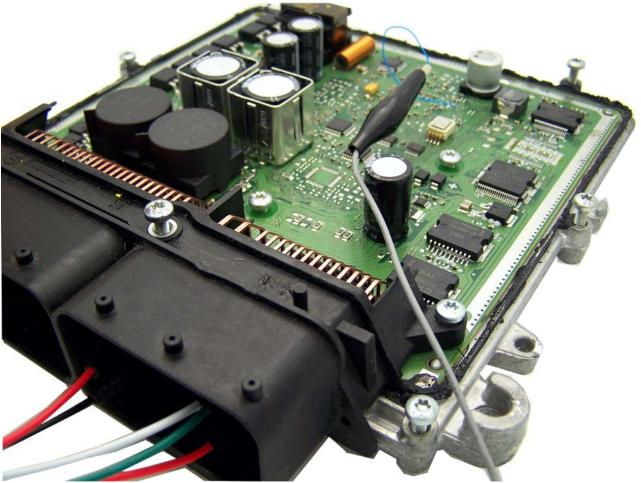
Figure 27 The DB15 Cable connections to Bosch EDC17 with the TC1796 MCU.
