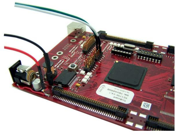
Figure 25 The DB15 Cable connections to Infineon TriBoard with the TC1796 MCU.
